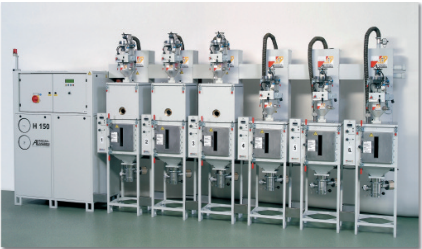
Drying bin is filled by an exact dosing of max. 4 components.
